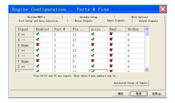
2) The tool and origin shall be controlled by input port. The tool works when connecting the tool detection.
